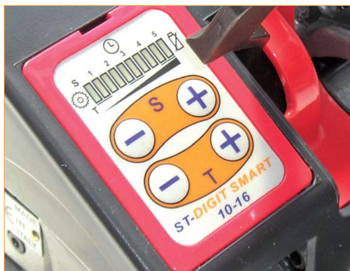
New digital adjustment system for tension and sealing time
